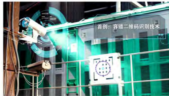
The FTIV, an innovative product for identifying hot metal ladle codes, has been applied successfully at WISCO
