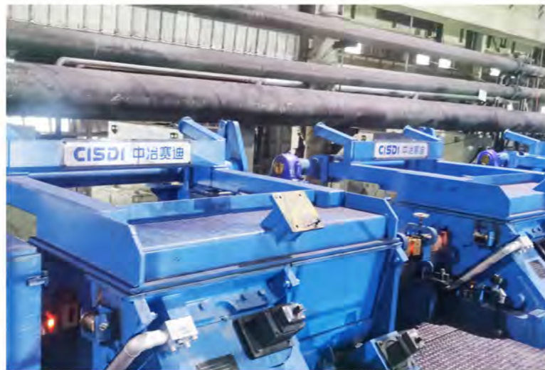
China's first modular Finishing Mill is now operational at Pangang Changcheng Special Steel's high-speed wire-rod rolling line. It was supplied by CISDI.
