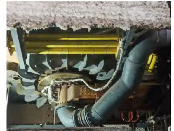
The air-cooled, feeler-pin bottom anode, to be installed at an EAF
