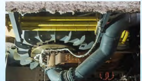
The air-cooled, feeler-pin bottom anode, to be installed at an EAF
