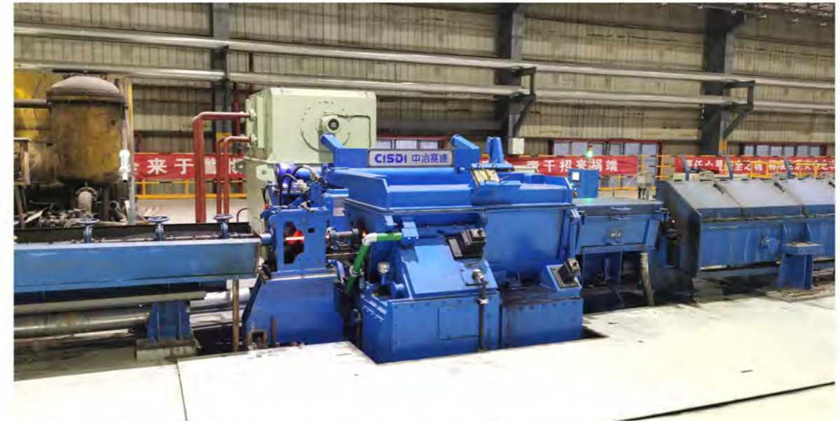
The SRSCD mills at Jianlong Ningxia's wire-rod rolling line operate at a speed of 100-plus metres per second
