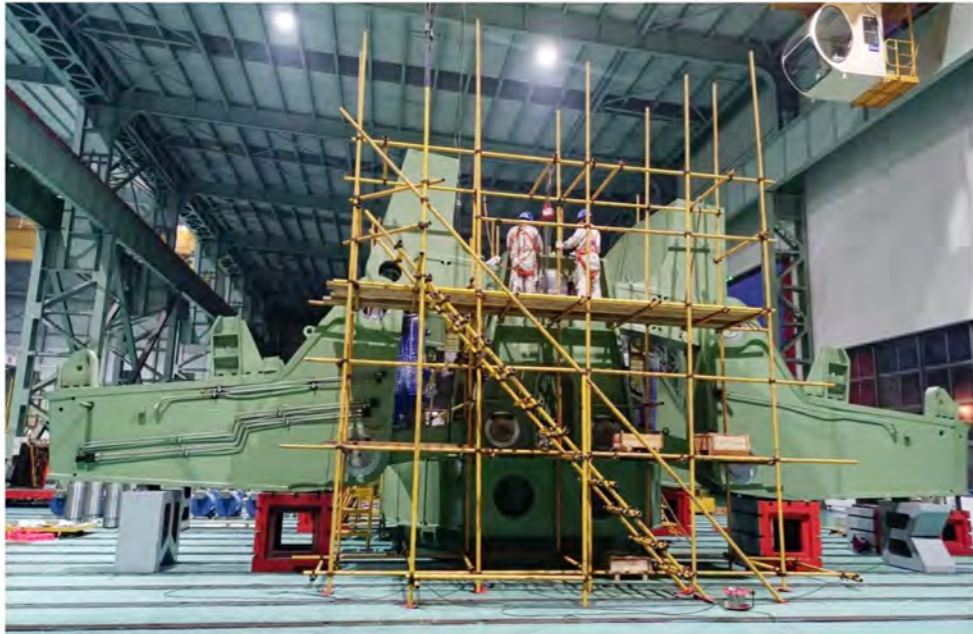
The challenging assembly of the ladle turret at CISDI Equipment Co's workshop
