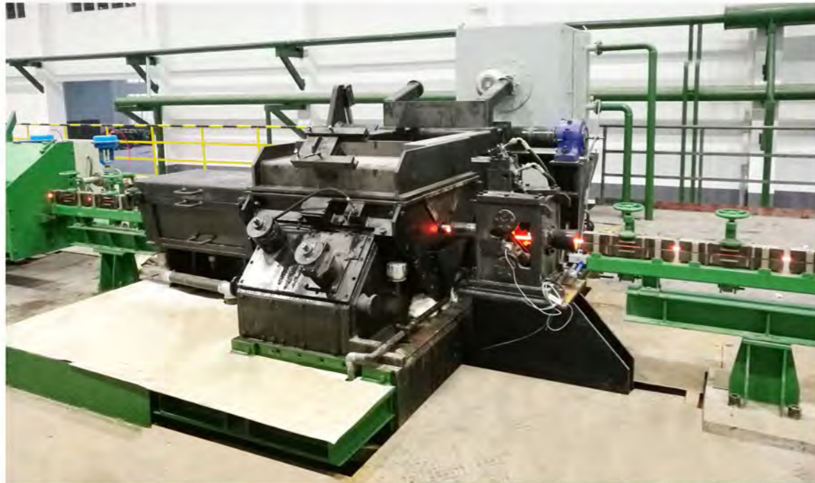
SRSCD mills operating at Yasheng's high-speed wire-rod rolling line
