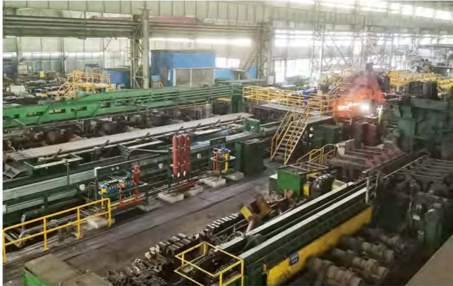
Hot testing of the three-roll cross tube mill, which now features an upgraded mandrel system
